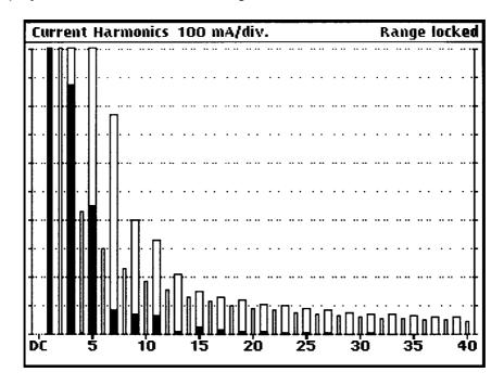
The horizontal scale is marked with the harmonic number. Odd harmonics & limits are shown as wide bars and even harmonics & limits are shown as narrow bars. The fundamental is shown to the left of the second harmonic as a wide bar and the DC component is shown to the left of the fundamental as a narrow bar.
